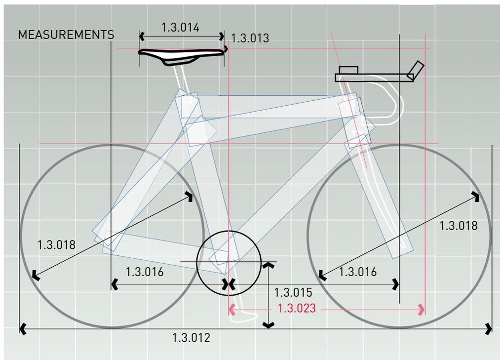
The profile of the extension must conform to the 1:3 ratio in accordance with Article 1.3.024. The extension must be fixed and not feature a system that would allow a change of length or angle during the race.
