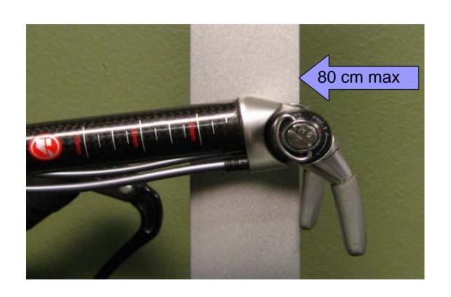
The bar is right at the 80 cm limit. The pivot of the shifter is the measurement point used.
