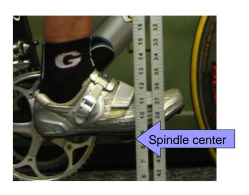
Locate the center of the spindle with the edge of the square.
