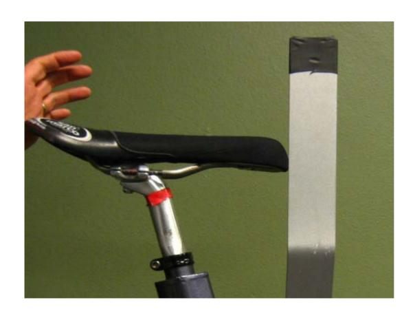
This saddle is 5 cm behind the bottom bracket. This position passes and does not require the morphological test for any event.
